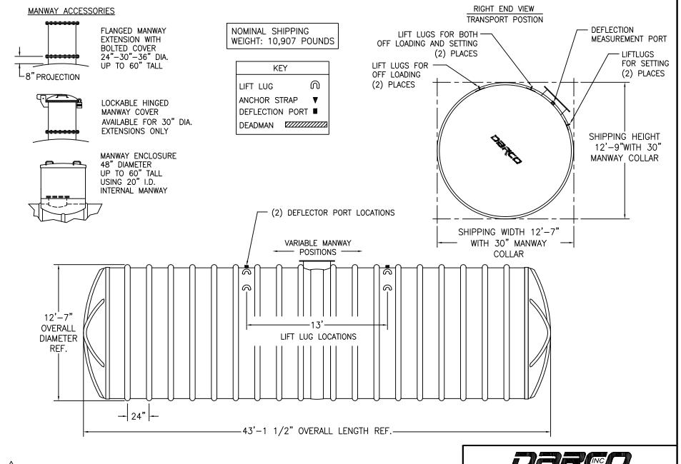
MINIMUM SOIL DEPTH ABOVE TANK WHEN USING DEADMAN ANCHORS IS 2 FEET.
