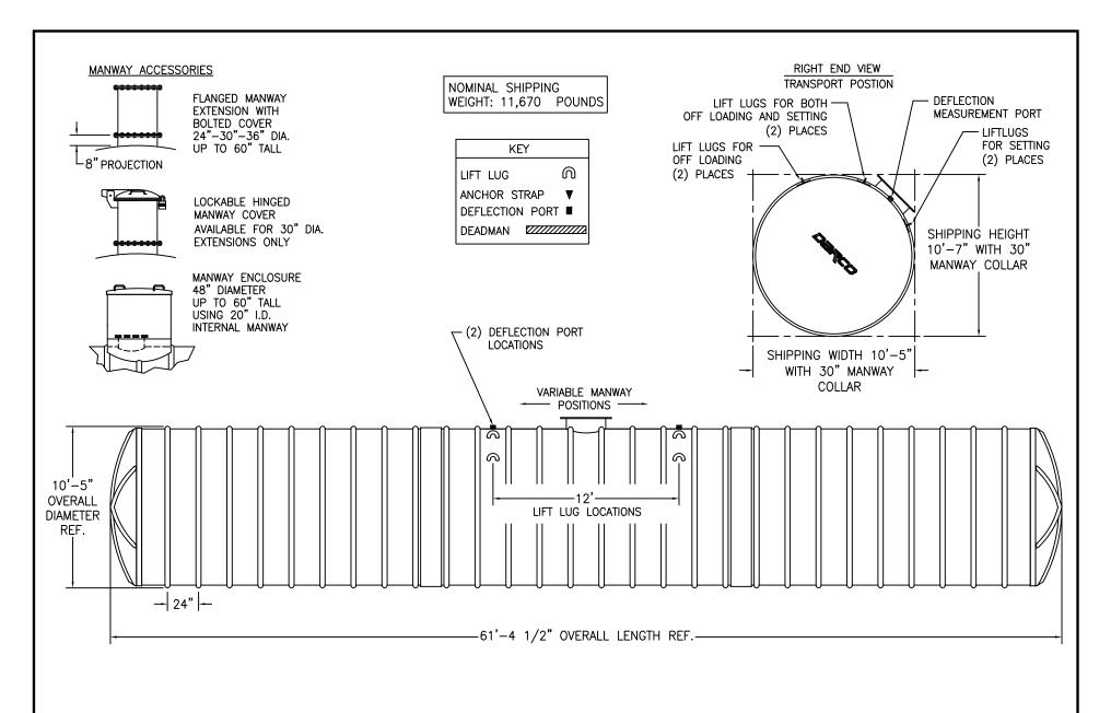
MINIMUM SOIL DEPTH ABOVE TANK WHEN USING DEADMAN ANCHORS IS 2 FEET.
