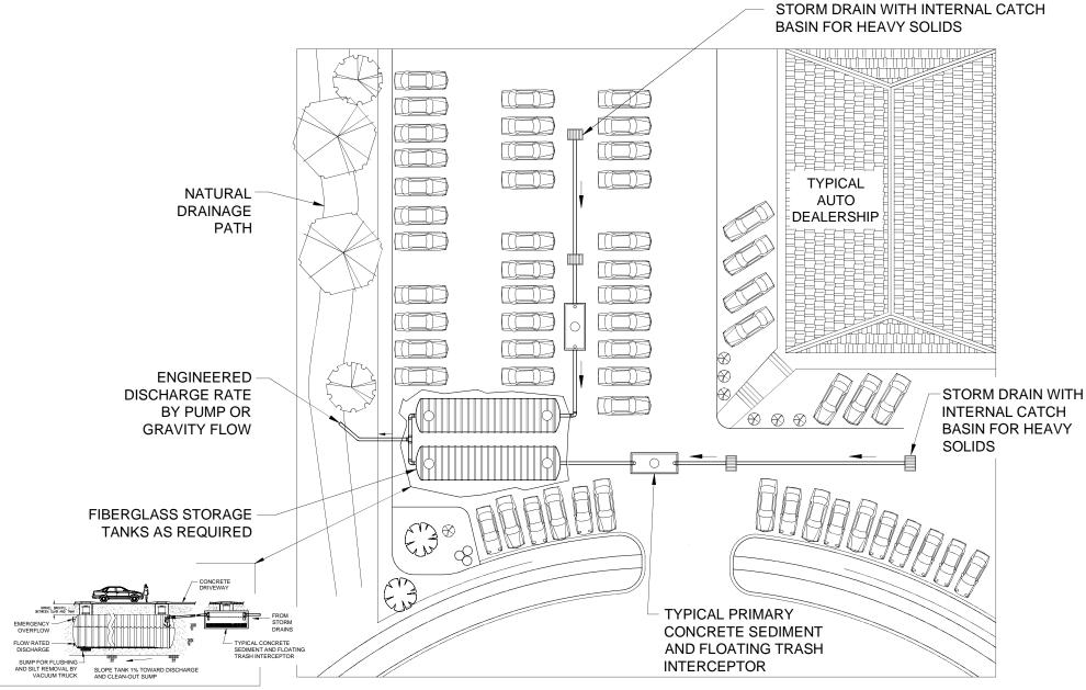
DETAINED STORAGE IN SINGLE OR MULTIPLE TANKS
